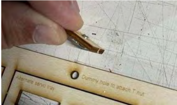
5. The T nut passes Through the former
